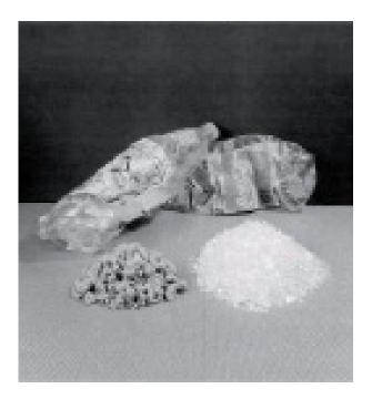
The tightly adhering labels on the otherwise clean material so far complicated the processing of this kind of plastics waste. Dry processing with air classifiers failed. Melting filters of a special construction type proved to be too complex. So one felt obliged to cut out the labels from the discarded material – an enormously time-consuming and expensive procedure, even disregarding the inevitable material loss.
