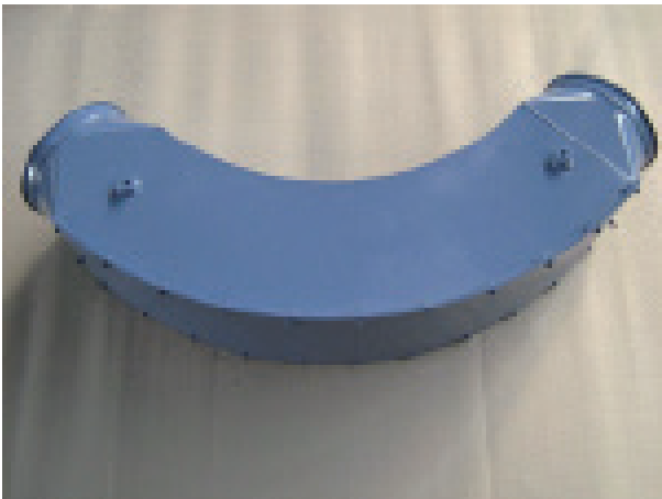
Fig. 1: The HERBOLD wear-resistant pipe elbows are prone to less wear than a traditional pipe elbow due to the larger radius.
