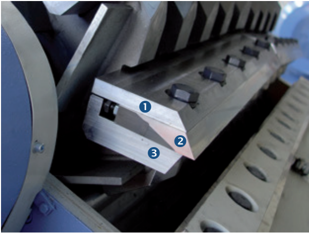
Fig. 3: ① Support plates for knives ② Rotor knives ③ Replaceable wear part
