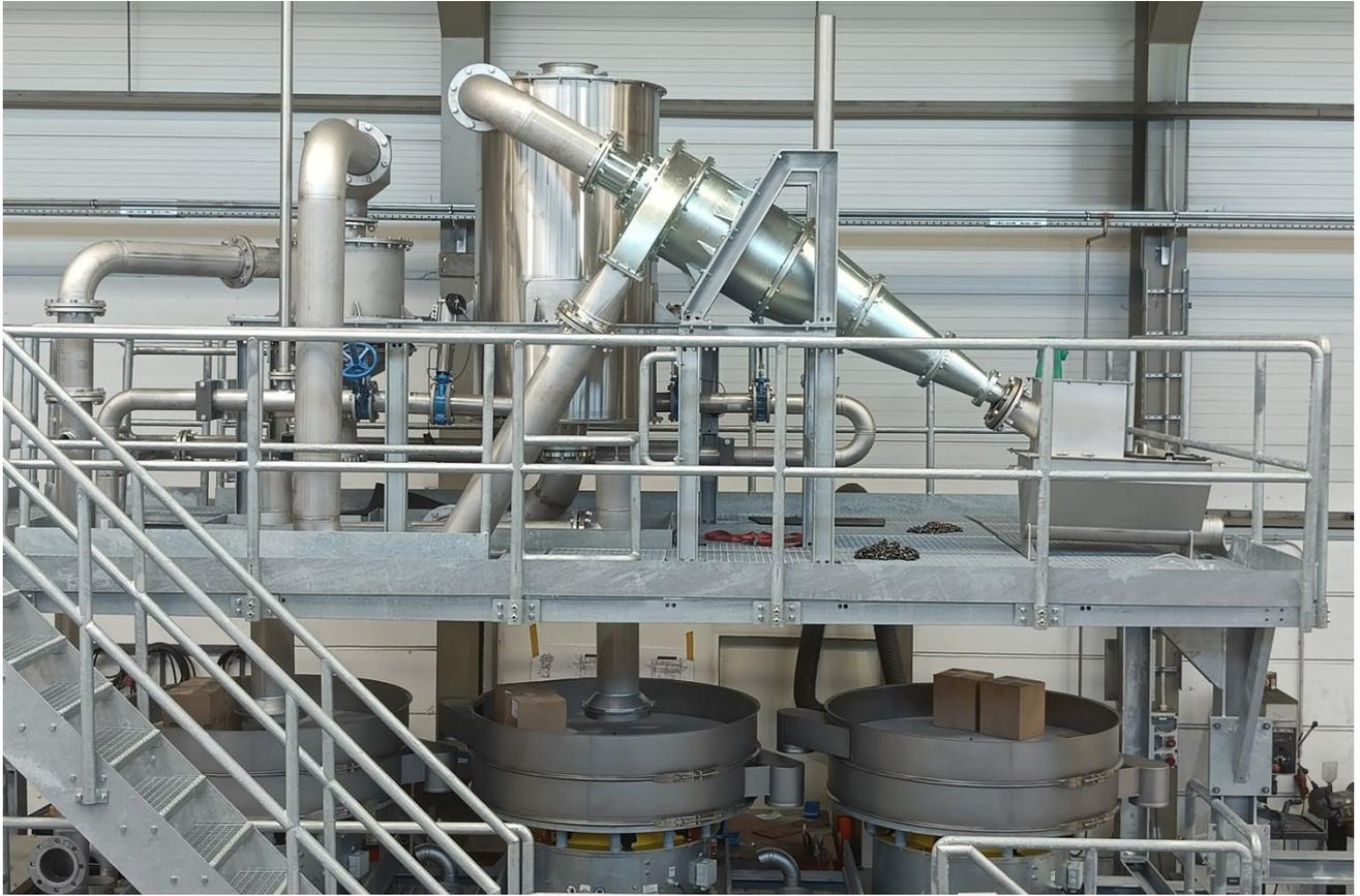
**Figure 3:** Like the entire PET recycling plant, the hydrocyclone stage for Dođa is designed for an output of 100 metric tons per day.
